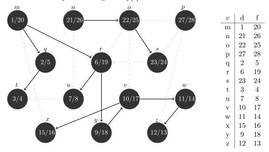
2. as each vertex is finished, insert it onto the front of the linked list
